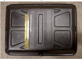
7. Drill holes on opposite side. I.E. If you drilled top left hole on the 5<sup>th</sup> divot down from the top, drill the top right hole on the correct divot line, in the 5<sup>th</sup> divot down, and repeat step 6.
