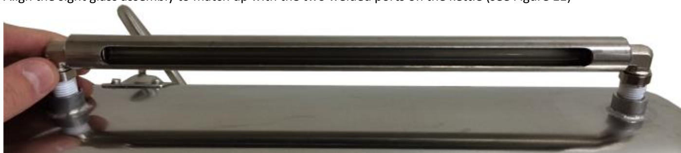
Figure 11 – Assembled sight glass aligned with welded ports
