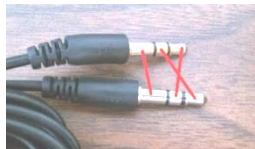
Bad ones are connected like this
