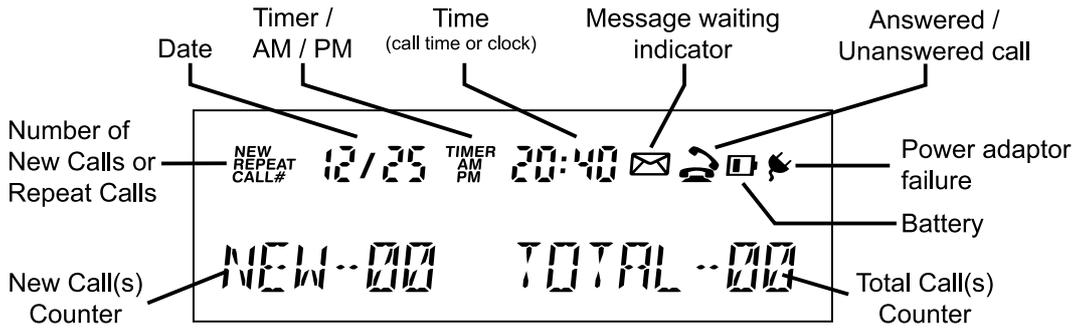
**FIGURE 3A: DISPLAY IN IDLE STATE**
