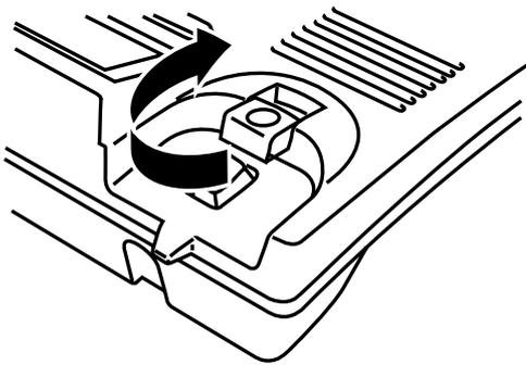
4. Insert the HANDSET RETAINER back into its slot
