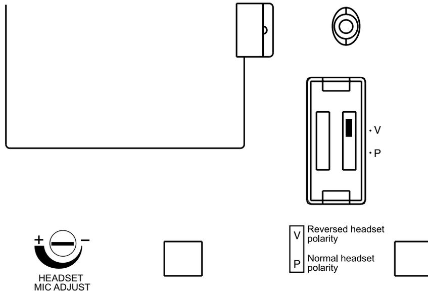
**FIGURE 7: HEADSET MIC ADJUST CONTROL AND POLARITY SWITCH**
