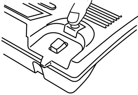
2. Push the HANDSET RETAINER out of the slot
