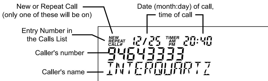
**FIGURE 5: DISPLAY OF A TYPICAL CALL FROM THE CALLS LIST**
