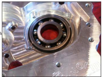
Discard snap ring from the support bearing for the idler gear. Gently tap bearing into bore in the center of the adapter with the snap ring groove up.
