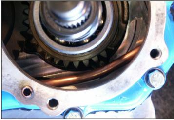
Swap bearing from original idler gear to modified gear by pulling snap ring and bearing, then cleaning and reinstalling onto modified gear. With idler gear in the cover or in the lefty silicone gasket surface and install cover on lefty.
