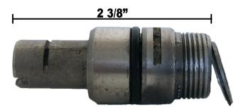
Glue cable drive housing into the Adapter with epoxy, total height should be 2 15/16". Be careful not to overdue the epoxy, its main purpose is sealing, not strength!
