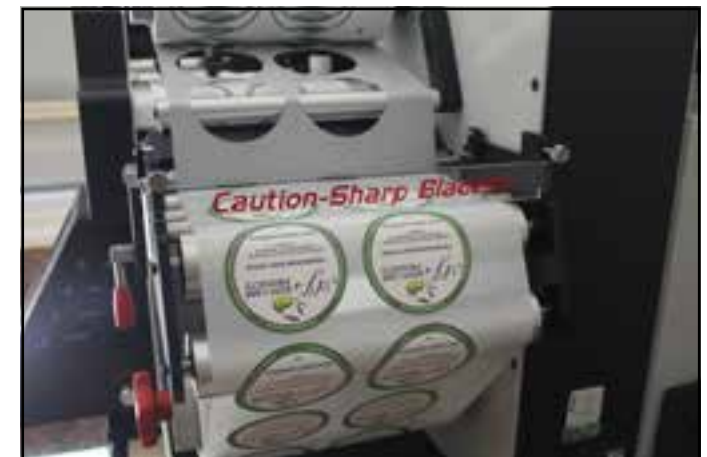
Excess label is removed and printed label wound onto roll
