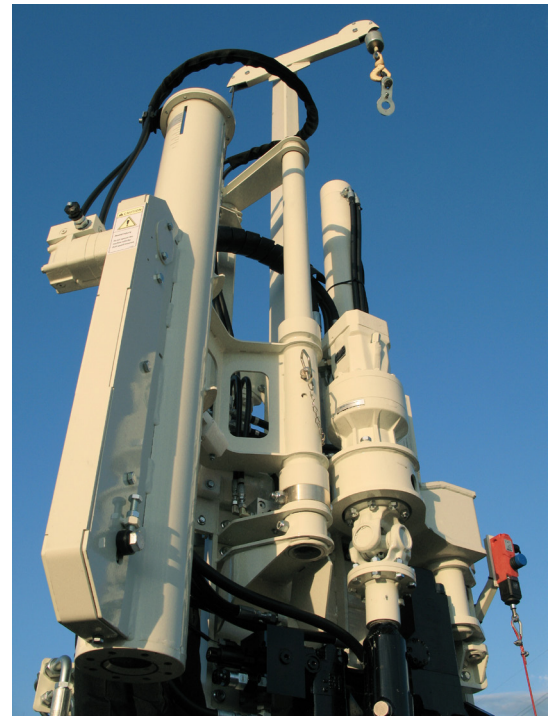
The DH103 Automatic Drop Hammer for the Geoprobe® 7822DT
