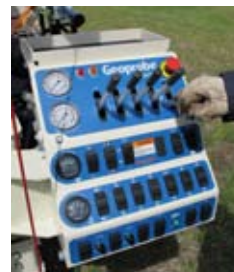
(above) Redesigned control panel provides more control and more feedback. (right) 7822DT features an industry-first integrated two-speed, bi-directional rotation with 225 to 450 ft. lb. of forward torque.
