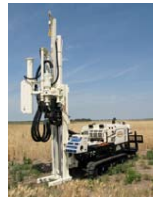
(above) Redesigned control panel provides more control and more feedback. (right) 7822DT features an industry-first integrated two-speed, bi-directional rotation with 225 to 450 ft. lb. of forward torque.
