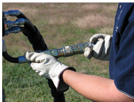
Hydraulic Quick Connects for easy & convenient set up and tear down of the 420M probe unit.
