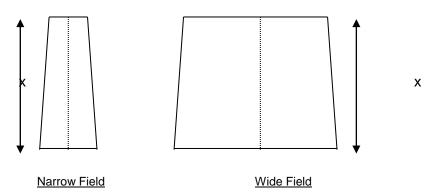
Diagram A illustrates this perspective problem, both fields are the same length but when on the approach the narrow field would feel and appear to have a longer run available than the wide field.
