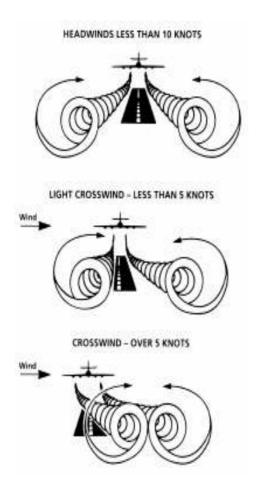
Close to the ground vortices generally persist for about 80 seconds. Here their effect is most hazardous. They tend to move apart at about 5 knots in still air, so a crosswind component of 5 knots will maintain the upwind vortex stationary on or near the runway. The downwind vortex will move away at about 10 knots. In a crosswind of more than 5 knots, the area of hazard is not necessarily aligned with the flight path of the aircraft creating the vortex.
