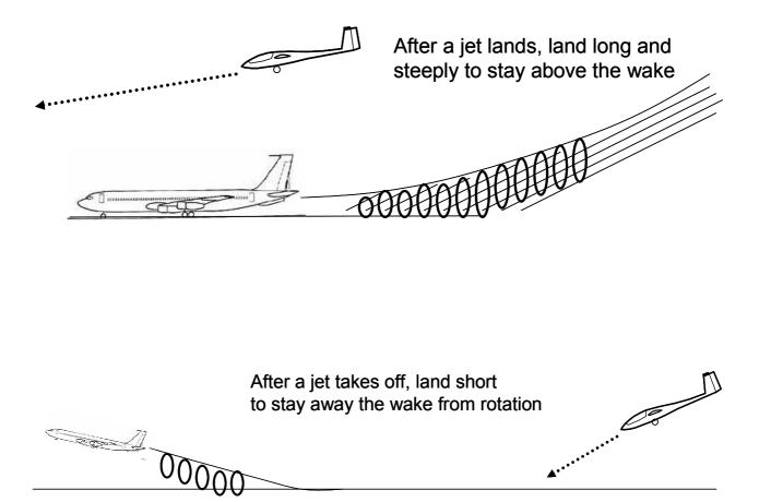
If you do not have to land during a movement, you should avoid doing this if possible. It only takes about three minutes for the whole vortex to dissipate. If possible, keep soaring for an extra three minutes between a departure and a landing or take-off to be sure the turbulence has ceased. If you are having difficulty in staying airborne, try to land well before the movement
