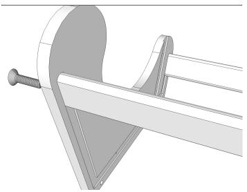
3. Insert the other End Board, with threaded insert, into the rear groove flush with the top of the groove. Secure End Board using a Flat Head Screw.
