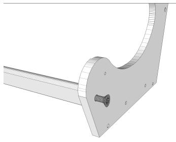
2. Secure the End Board to the right Side with a Flat Head Screw.
