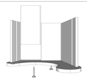
6. Place the Middle Boards into the remaining horizontal groove and secure with two Wood Screws.
