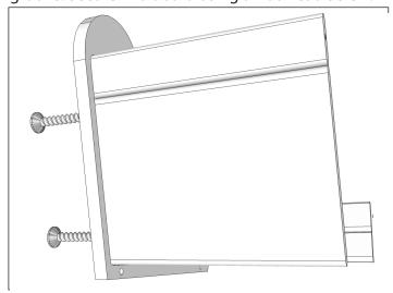
5. Place Lower Head Board into horizontal groove securing with two Wood Screws.
