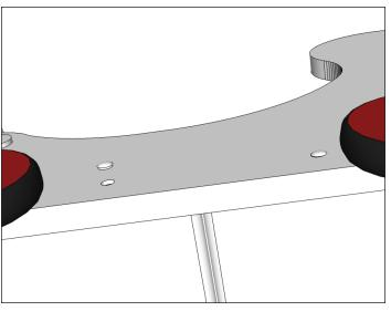
12. Insert Button Caps into screw holes in by placing a dab of glue on their ends and pressing down or lightly tapping with a hammer.
