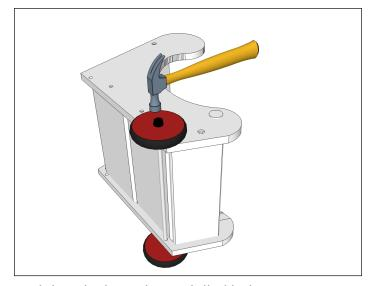
9. Slide Axle through pre-drilled holes in Pram, turn over and slide opposite wheel onto the axle (smooth side out). Secure Axle End Cap with a hammer strike. Repeat steps 8 and 9 for other Axle.
