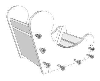
7. Fully seat Left Side on top of Pram assembly. Secure End boards with Flat Head Screws and Middle and lower Boards with Wood Screws.
