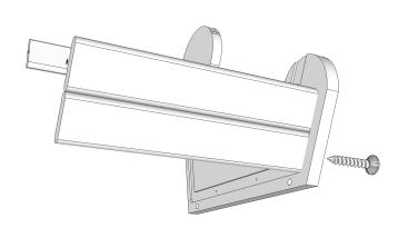
4. Place the Lower Foot Board underneath the End Board, secure using a Wood Screw.
