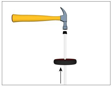
8. On a sturdy hard surface place Axle End Cap on the end of Axle, seat with a hammer strike. Slide a wheel (smooth side out) onto Axle.
