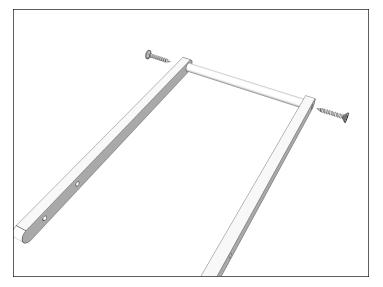
10. On a flat Level surface place Handle into predrilled holes in the Handle Arms. Ensure the assembly is square and secure using Wood Screws.
