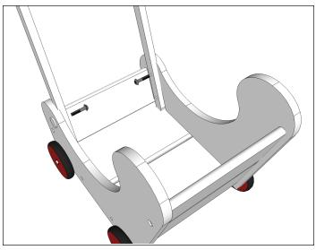
11. Place handle assembly into the grooves in the Pram and desired handle height. Lower position is 21" and upper 24" from the ground. Secure with two Chicago Bolts.
