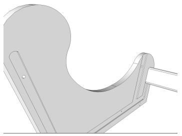
1. Insert one End Board into the front groove on the Right Side ensuring the rounded edge is flush with the top of the groove.
