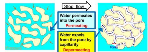
Figure 6. Schematic diagram of C18 particle
