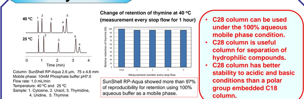
Figure 8. Separation of nucleobases and retention time stability
