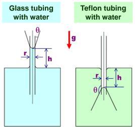
Figure 7. Schematic of capillarity
