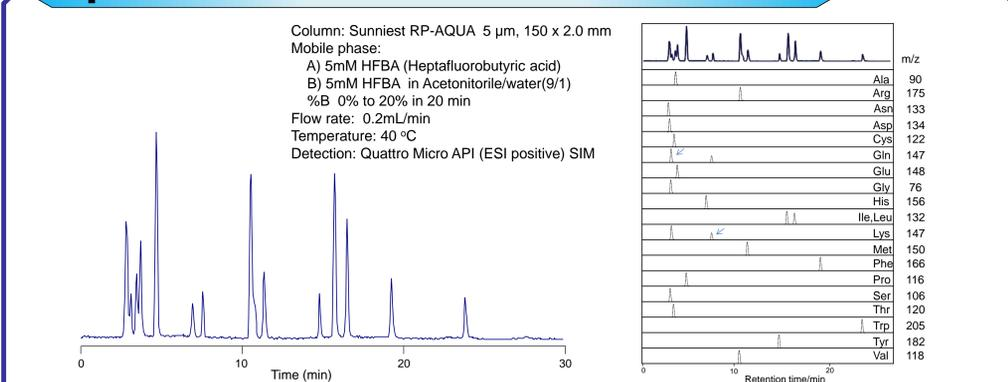
Figure 10. Separation of amino acids using UV and MS detections
