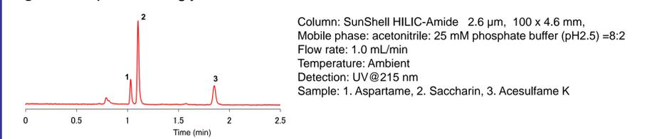
Figure 5. Separation of synthetic sweeteners
