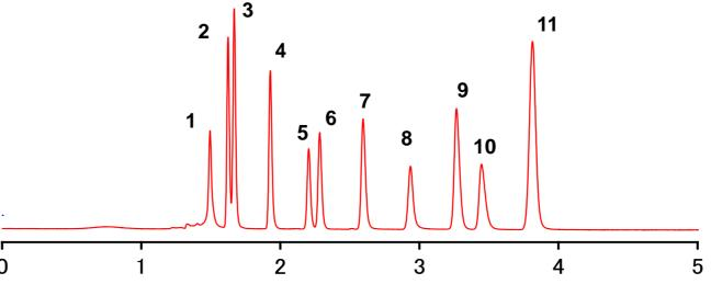
Column: SunShell RP-AQUA 2.6 µm, 150 x 4.6 mm Mobile phase: 0.025 M KH2PO4, pH2.5 Flow rate: 1.0 mL/min Column pressure: 32 MPa for 1.5mL/min Temperature: 40 °C Detection: UV@210nm Injection volume: 2 µL
