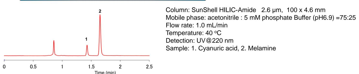
Figure 3. Separation of melamine and cyanuric acid
