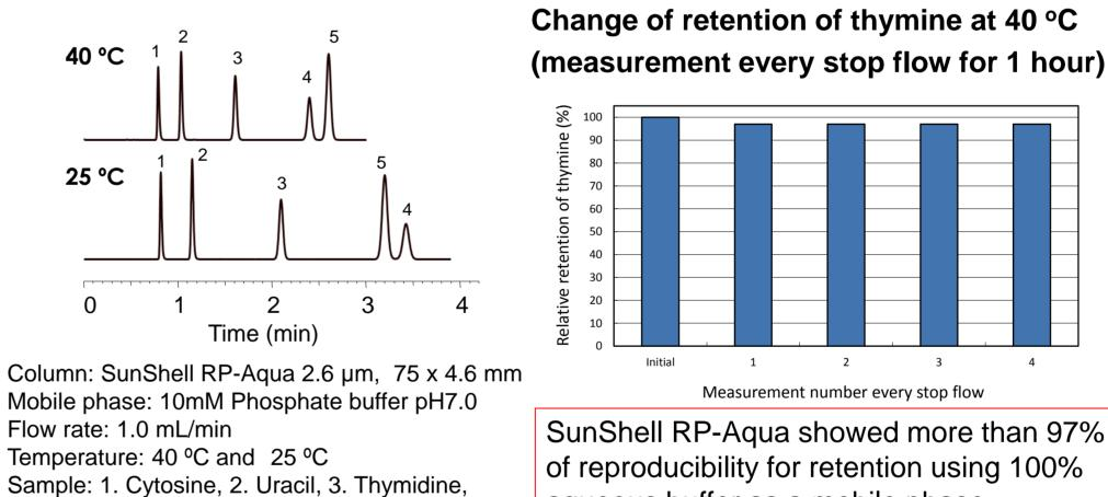
of reproducibility for retention using 100% aqueous buffer as a mobile phase.
