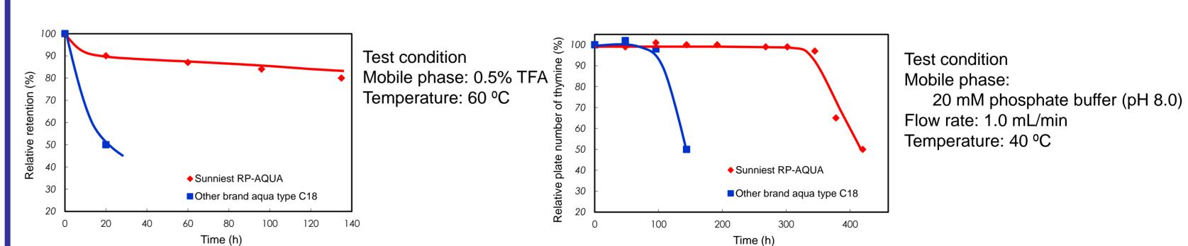
Figure 9. Stability of C28 under acidic and basic conditions
