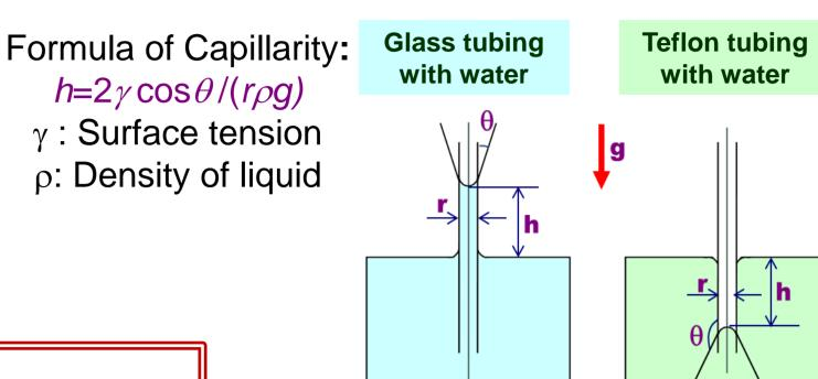
Figure 7. Schematic of capillarity
