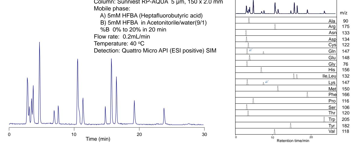
Figure 10. Separation of amino acids using UV and MS detections
