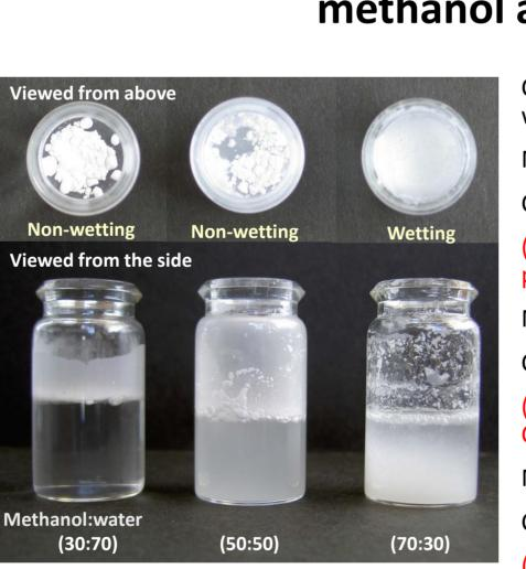
C18 packing materials were put into each solvent and stired with ultra sonic vibration.
