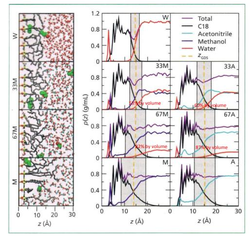
Mark R. Schure et al. reported the left figure . A bonded phase collapses under methanol:water=53/47(v/v) as well as under water.
