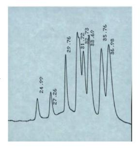
Excellent separation was obtained in 15 minutes when the oligonucleotide standard, oligothymidylic acid d(pT) 12-18 mer, was chromatographed using the nucleic acid column. The larger oligonucleotide fragments may be purified by adjustment of elution conditions. They require higher concentrations of salt and longer times for elution.
