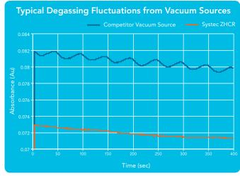
Fluctuations in detector baseline of a single-speed pump compared to the patented technology of the Systec ZHCR vacuum pump.\* UV detector baseline fluctuations are minimal when compared to traditional stop and start vacuum sources.
