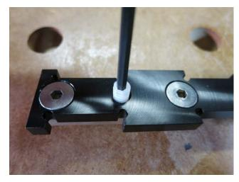
The narrow stock adapters are designed to interlock with the tail brackets: Interlock these two parts and slide them both on to the Incra T-Track. Once assembled, this allows accurate positioning of the short stock adapters using the Incra T-Track scales
