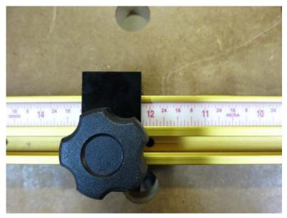
8. Alternatively, if you don't require the scales to direct read, you can use a tape measure to position the rail stops relative to the saw cut line.
