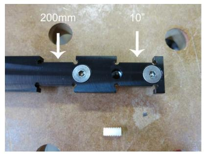
The nylon set screw allows positioning of the narrow stock adapters from the bottom of the Incra rail for even more precise measurements. To use this way, simply measure and position the narrow stock guides using a rule, and use the set screw to hold the narrow stock adapters in place.
