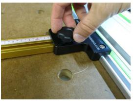
3. Slide the rail stops onto the Incra T-Track Plus.
