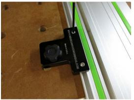
2. Install the Incra T-Track Plus into the rail bracket adapters with the included knob/hardware. Note that the knob can be inserted in either of two holes to allow positioning the T-Track Plus on either side.
