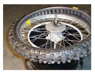
10) Use long tire irons to force the remainder of the first bead over the rim flange.
