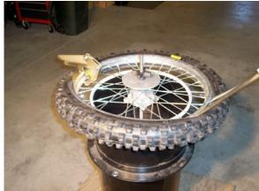
Once the tire bead is stretched tightly and it becomes difficult to insert the tire iron between the tire and rim, use a tire iron adjacent the bead hold down clamp to force the first portion of the tire bead into the rim recess area.
