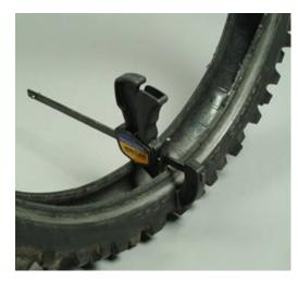
5) Insert fully inflated Tire Balls<sup>™</sup> into the tire carcass pressing them against the quick clamp. Make sure that the inflation inserts are all facing the same direction.
