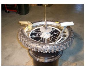
13) After removing the Bead Hold Down Clamp, attach an inflation hose to the valve stem (core removed) and inflate to seat the tire beads onto the rim.
