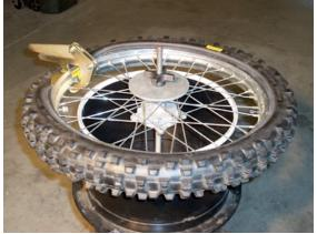
12) Once the motorcycle Bead Hold Down clamp is in place, long tire irons can be used to force the remainder of the tire bead over the rim.
