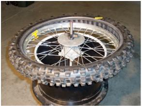
11) Force the tire down onto the rim so that the remaining tire bead is lying next to the rim flange. Next position the Bead Hold Down clamp in between the closest parallel spokes to the rim lock. Take 2 tire irons and lever a section of the tire bead over the rim flange so that the Bead Hold Down clamp can be locked into position, a small amount of bead lube smeared between the clamp and tire makes the installation process easier.
