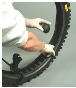
6) Install as many Tire Balls<sup>™</sup> into the tire carcass as will fit. Typically, the number required will be 35-38 Tire Balls<sup>™</sup> in a front (in kit of 40) and 24-28 in a rear tire (in kit of 30)
