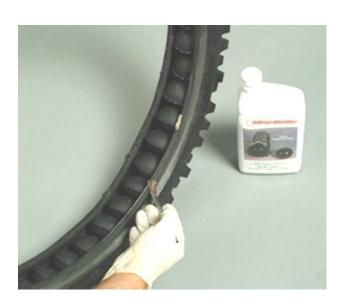
9) After checking and aligning for tire direction and wheel direction, force the first tire bead over the rim flange starting at the rim lock. Force as much as possible by hand before picking up the tire irons to complete this step.
