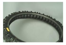
7) If you intend to raise the pressure above the preset psig, then bring each ball up to the final pressure gradually, alternating between every other ball, much as you would torque a cylinder head, using the inflation regulator and pressure gauge. The intent is to inflate the balls so that they are the same size and pressure.
