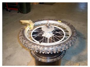
14) Remove the remote inflator, install the valve core and cap; tighten the rim lock nut. The tire is now ready for mounting on the vehicle.
