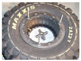
10) After removing the Bead Hold Down Clamps, apply additional bead lube onto the exposed tire bead and rim. Laying the wheel flat on the ground, attach an inflation hose to the valve stem (core removed) and inflate to seat the tire beads onto the rim.
