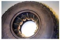
6) Lubricate the rim with the water-based tire bead lube as well as the tire beads.
