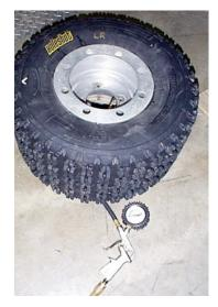
For your own personal safety, never use an air chuck applied to the valve stem, use a remote inflator as shown.
