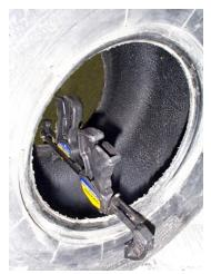
4) Install Tire Balls<sup>™</sup> into the tire carcass in a partially inflated state. Typically, the number required will be 12-14 Tire Balls<sup>™</sup> in either a front or rear ATV tire. Contact us at 877-847-3225 for exact recommendations for your particular brand tire and wheel.
