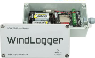
LeWL windlogger has been designed for small scale wind assessment with no need for a computer to log data. It is a completely stand alone system. The unit shares many features from the professional wind energy world such as providing average, standard deviation and gust wind speeds recorded every 1 minute or 10 minutes. The LeWL windlogger is fully configurable to select between one or two simultaneous anemometer readings with changeable conversion factor to calculate wind speed.
