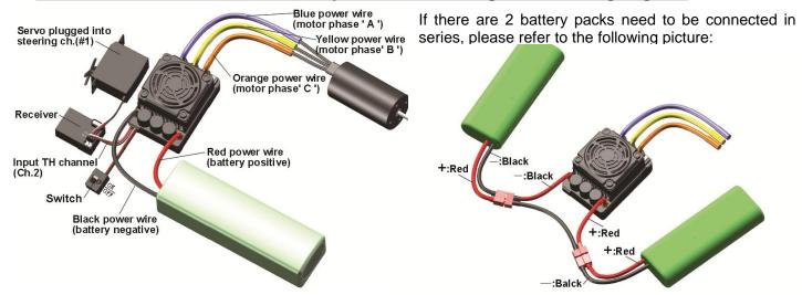
**Note3:** There is a small female connector that coming out from the "FAN" socket, this is used for connecting with the cooling fan of the brushless motor.
