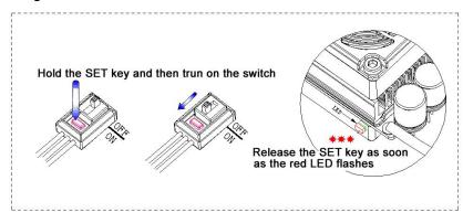
Note4: If you don't release the "SET" key after the red LED begins to flash, the ESC will enter the program mode, in such a case, please switch off the ESC and re-calibrate the throttle range again from step A.
