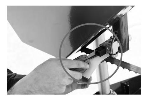
Using a 6mm allen key, loosen the blade guide blocks on both the left and right sides. They should be free to slide up and down.
