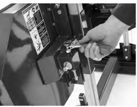
To adjust the left side of the sawmill, again start by taking the tension off of the blade by turning the "T" handle one turn in the counter-clockwise direction. Using a 16mm wrench, loosen the "vertical nut" a ½ turn. Do the same on the "bottom vertical nut". Next, loosen both "vertical bolts" a ½ turn. This will take the clamping force off of the bandwheel shaft caused by these two bolts and allow it to move freely in the following steps.
