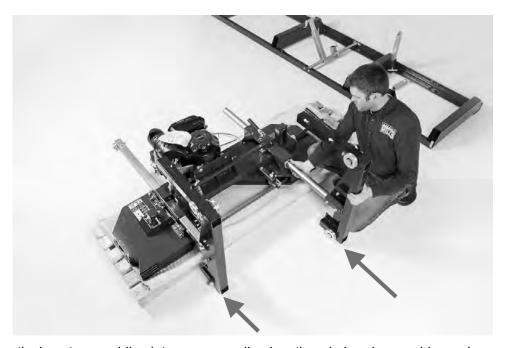
Insert vertical post assemblies into corresponding locations in head assembly as shown above.
