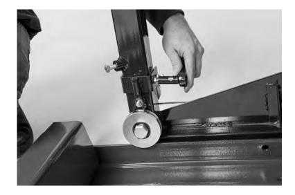
Attach the four track sweepers to the frame so that the steel brush reaches the bottom of the groove in the carriage wheels. Use a 13mm socket to fasten.
