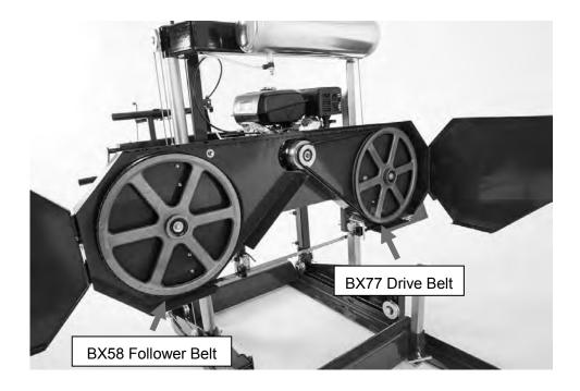
There are two rubber "V" belts on the sawmill and they should be replaced as a set. It is not advised to replace individual belts separately. It is recommended to to use a BX77 cogged belt for the drive side and a BX58 follower belt.
