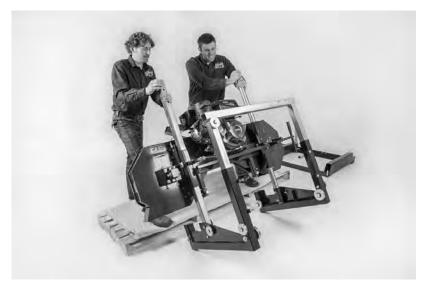
With one person on each post, stand the head assembly up on the wheels as shown above. Again, using a **minimum of two people**, set the saw head assembly on the track system ensuring the carriage wheel grooves rest on the "L" rails. The square vertical post should be on the same side as the log supports.
