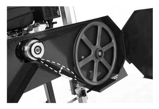
To check the belt tension, with your hand, firmly try to deflect the belt up and down. There should be no more than 1/4" of deflection in both directions (1/2" total). If the belt deflects more than this, it will need to be tightened as described below.
