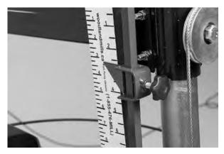
Slide the scale indicator over the square rod and tighten.
