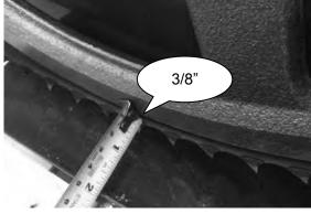
Re-tension the blade by turning the "T" handle a full turn in the clockwise direction. Wearing gloves, spin the bandwheel with your hand and observe how the blade has changed tracking. Measure the distance again and repeat the above step to further compensate if required. The ideal measurement is 3/8".
