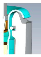
However, the ridge in a standard filter serves a purpose. It's designed to work with the spring clip (see image) and serves to pull the filter all the way down into the portafilter housing and hold it there. Notice the placement of the spring clip that fits into the portafilter groove; in a properly designed filter, it lands precisely against the top radius of the ridge. Some users have both Standard and Ridge-Less styles in their favorite sizes (dose capacities).
