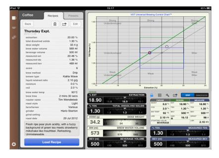
To load the selected and displayed recipe click the "Load Recipe" button, and the brew parameters will snap to the original design values of the recipe, and computed values will be updated in the dashboard panel.
