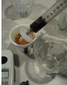
Place the syringe tip under the Attach a syringe filter approx a quarter-turn until snug. Do not over tighten.
