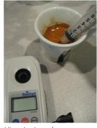
Allow 1 minute for espresso to cool and CO2 to diffuse out of solution. Stir the sample.
