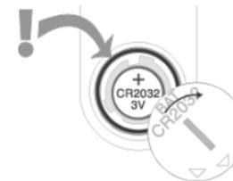
Replacing the Battery
