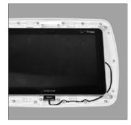
**3.** Plug the charge and sync cable into your tablet's charge port, then place your tablet inside the enclosure face up.
