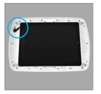
**NOTE:** Here's an iPad installed in the correct orientation with the Power Button Trigger next to the iPad's power button.
