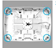
2. Place the head unit onto a clean surface with the inside of the enclosure facing up (your charge and sync cable should be on the right side of the enclosure as shown in the photo). Slide all four of the green retaining clips towards the outside of the enclosure.
