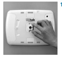
**1. Open the lilitab head unit** by placing it facedown on a clean surface and squeezing the finger latches together as shown. Carefully lift up and the faceplate will release, allowing access to the inside of the head unit.
