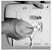
4. Install the charge and sync cable that came with your tablet into the head unit by threading it through the metal plate located in the center of the head unit.
