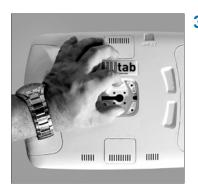
3. Open the lilitab head unit by placing it facedown on a clean surface and squeezing the finger latches together as shown. Carefully lift up and the faceplate will come off, allowing access to the inside of the head unit
