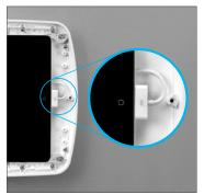
**6.** Plug the cable that came with your tablet's into it's charge port and place it inside the enclosure face up (screen faces towards you).
