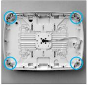
5. Place the head unit onto a clean surface with the inside of the enclosure facing up (the lilitab logo on the rear of the unit will face down and away from you). Slide all four of the green retaining clips towards the outside of the enclosure.
