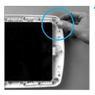
7. Slide all four green retaining clips towards the center of the tablet ensuring they securely hold the tablet in place.
