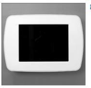
8. Position the faceplate over the tablet such that its openings are oriented as you wish (faceplates have different combinations of home button and camera openings). Gently press down around the edge of the faceplate and it will snap into place.
