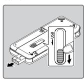
3 Make sure that the recorder is in stop mode, and connect to the PC's USB port.
