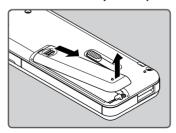
Insert the battery, observing the ⊕ and ⊖ polarities.
