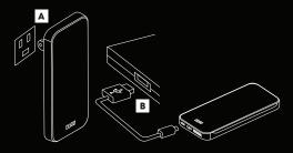
It takes approximately 5-6 hours to fully charge your Pocket Julice Charger (from depleted unit). Once the charging is in progress, the Indicator Lights will illuminate accordingly (see charging chart above).
