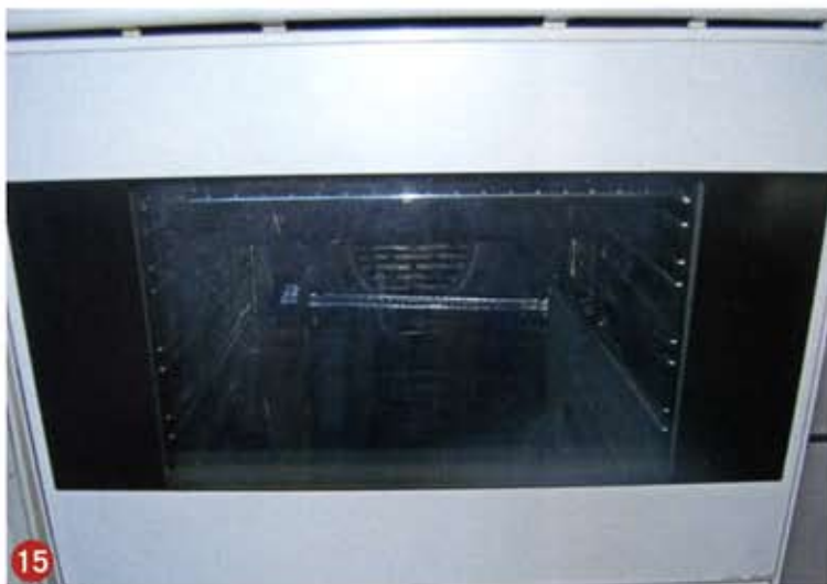
▲ The oven is set to 180deg C. When the powder melts to a gloss finish, start timing. It needs 10 minutes to fully cure.
