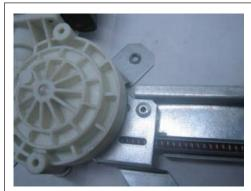
Drill rivet located at bottom of track.
