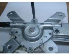
2. Remove three torx drive screws, holding the motor and remove motor. Remove worm drive from track as well.
