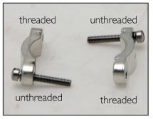
Each half of the clamp connector has a threaded hole and a non-threaded hole. Put the screws through the non threaded hole first, then screw into the threaded hole to hold the clamp connector in place.
