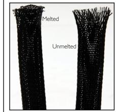
Cut Ultra Wrap to desired length. Melt the ends of the Ultra Wrap with a flame to prevent fraying and extend its life.
