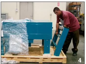
Remove the shrink wrap ( Photo 3). Then remove the Belt Extentions. DO NOT RE-MOVE THE SHRINK WRAP on the Belt Extentions these hold the Belt Rollers in place (Photo 4).
