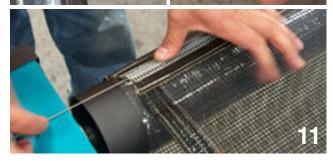
Join the two ends of the Belt by interlocking the ends an then feeding the Joining Pin all the way through (Photo 11).
