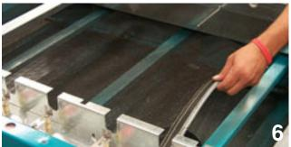
Keep feeding Belt back through the Heat Chamber staying on TOP of the Heat Chamber Braces (Photo 6).
