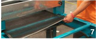
Pick up the other end of the Belt and lay on top of the ROLLER and pull the two ends of the Belt as close as you can get them (Photo 8).
