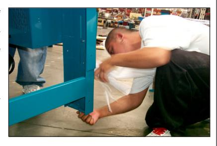
DO NOT try to raise the level of the Dryer with the Stabilizing Bolts and DO NOT use casters on the Dryer legs as this will cause damage to the metal structure. If the Dryer is not level lift the Dryer leg that will make it level before you attempt to adjust the Stabilizing Bolt.
