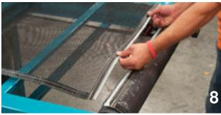
If the Belt does not fit together loosen the Tracking Bolts at the two ends of the Belt Extensions and then push the ROLLER in till you can join the two ends of the Belt (Photos 9 and 10).
