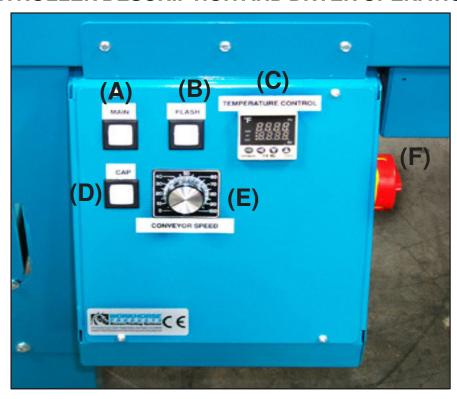
Before turning the Dryer on make sure that all objects are off the belts and all of the switches on the front panel are off or in the down position.
