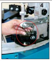
Step 5 Attach Springs / Ph 5/6 Once you have both sets of Springs and Hog Rings in place pull down the Print Head all the way so you can see through both UpStop Bolt holes, install stop bolt , then the nut and tighten by HAND not with a wrench (Photo 5)
