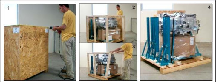
The WORKHORSE Mach Series Screen Press 4/4, 6/4, 6/6, 8/6, 8/8) Ships in one wooden Crate (Photo 1). Uncrate using a power Screwdriver (Photo 2). The 2x4 inner supports are nailed so you can just bend them to remove them. (Photo 3). The Finished Uncrating (Photo 4).
