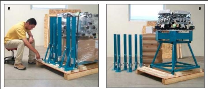
To remove the Print Arms from the pallet, use a 1/2" socket wench and unbolt them. (Photo 5). Mach Series Press with Print Arms, Shirt Boards and Small Parts Box removed .(Photo 6)
