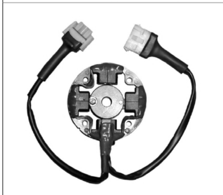
SELETTRA IGNITION (4 poles Digital) - IAME Part # 10015A
