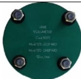
Cylinder Head CC Plate IAME Part # 10277
