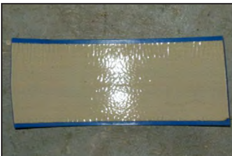
Sticky side of aisle stripe prior to adhering the sample to the floor.
