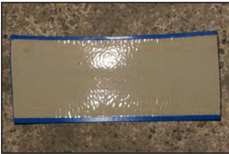
Sticky side of aisle stripe prior to adhering to floor.
