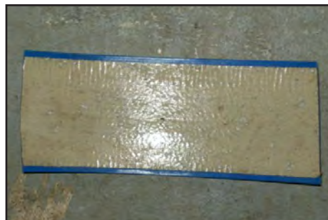
Sticky side of aisle stripe after adhering sample to a new sealed concrete floor. Floor was only swept clean. Adhesion was good but not the best. Note the contaminants on the adhesive.
