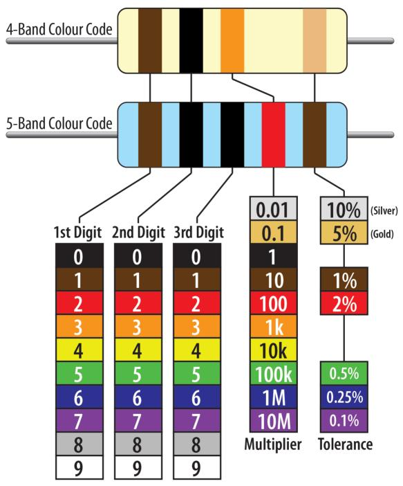
In the example, the 5-band resistor has the first band brown (1), second band black (0), third band black (0), 4th band is red (x100 multiplier), so the resistor value is 10,000 Ohms: usually written as 10k.
