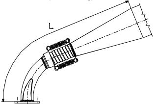
To achieve this dimension, the flexible (supplied with the engine) must be cut at a lenght of 65mm (flexible completely closed).
