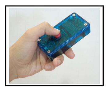
The BlueReader HF is a compact, affordable, handheld HF RFID reader. BlueReader contains a Bluetooth wireless link for easy integration with mobile phones. Bluereader contains a USB interface and high-capacity memory card that also enables it to be used as a stand-alone reader.
