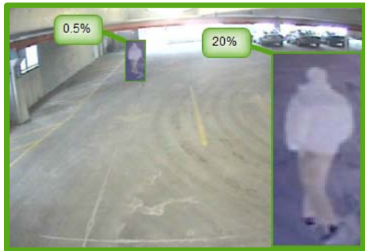
Figure 3. MORE EFFECTIVE – Two targets within the detection range taking up 0.5% and 20% of camera view
