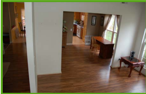
Figure 21. MORE EFFECTIVE – The camera is facing the interior of a home, mounted above the front door. The height and angle of the camera are optimal for event detection. Note that the camera must be high enough to not show the swinging door below.
