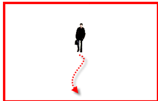
Figure 5. LESS EFFECTIVE – A target moving directly toward the camera spends less time in the camera view.
