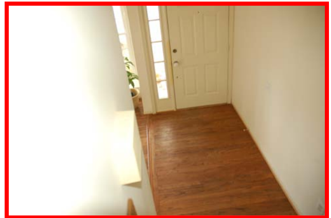
Figure 22. LESS EFFECTIVE – The camera is facing the door and covers a narrow view, so targets may not be in the scene for enough time (see page 4).
