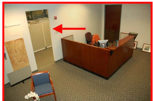
Figure 32. LESS EFFECTIVE – The camera view unnecessarily includes a doorway leading to the inside of the suite. Any activity in the walkway behind the doorway could trigger events.
