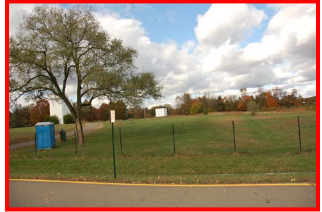
Figure 46. LESS EFFECTIVE – The camera is directly facing the fence, which means that people climbing the fence will be moving directly away from the camera.
