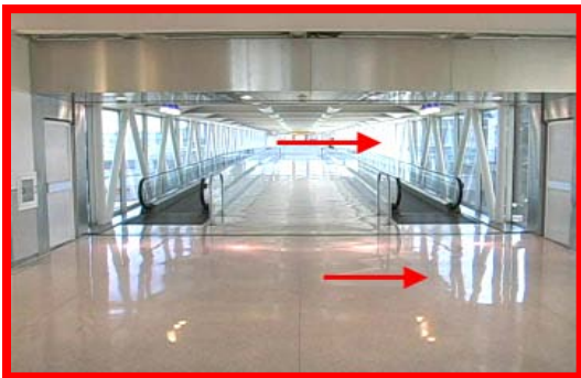
Figure 19. LESS EFFECTIVE – Windows and polished floors provide abundant reflections.
