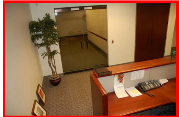
Figure 30. LESS EFFECTIVE – The camera is directly facing the glass door at the entrance, which can lead to reflections and unwanted event notifications (see page 7).
