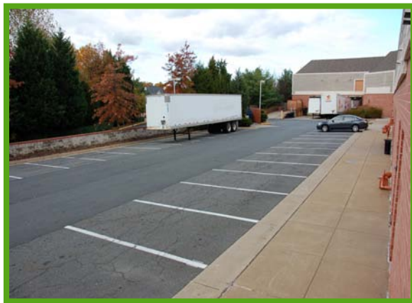
Figure 33. MORE EFFECTIVE — In this example, the camera is placed to monitor people approaching the building from the left side of the scene. The camera view covers a wide view of the building exterior while minimizing the wall it is mounted on.
