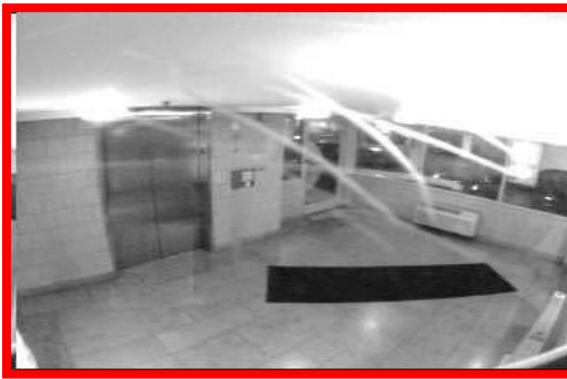
Figure 17. LESS EFFECTIVE – Example of light adversely affecting the camera view.
