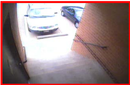
Figure 16. LESS EFFECTIVE – This scene includes too much contrast between the darkened hallway and the glare of light from the outside.
