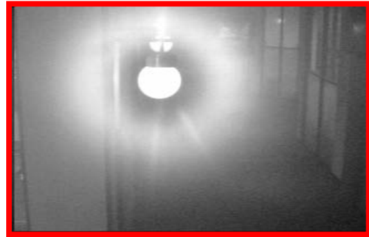
Figure 18. LESS EFFECTIVE – Light completely obstructing the camera view.
