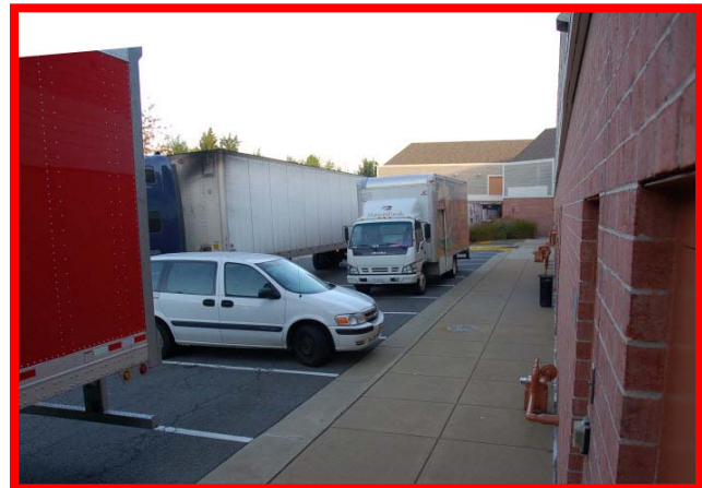
Figure 35. LESS EFFECTIVE — Several parked vehicles obstruct the camera's view of the entire scene, decreasing the amount of time a person would be visible.
