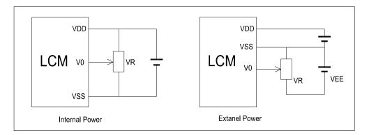
V<sub>DD~</sub>V<sub>0</sub>: LCD Driving voltage VR: 10k~20k
