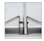
• Place the drilled plate in between the 2 pieces of metal base.
