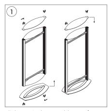
• Fix by screwing bottom and then top plates to side coloumn on both sides.
