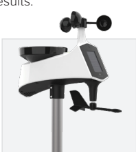
Freestanding Pole Setup 1" Maximum Outside Pole Diameter
