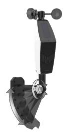
1. Install the Hand Screw to the bracket, then Secure the Glide Sensor to the Mast by tightening the screws on the side. This configuration allows you to attach the sensor to angled locations and easily adjust ensure the Mast and Sensor are level.
