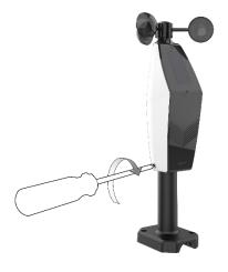
1. Secure the Glide Sensor to the Mast by tightening the screws on the side.
