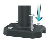
2. Mount the Mast to a flat surface with the four provided screws.
