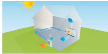
In summer heat is removed from the inside and vented to the outside.
