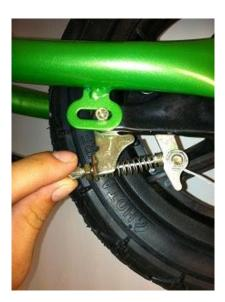
If the brake is too tight after you have turned the barrel adjuster clockwise all the way in or too loose after adjusting barrel counter clockwise all the way out, the cable will need to be adjusted.
