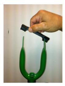
Insert the wheel into the fork and replace the hook washers onto the axle so the tab fits into the corresponding hole, then put on flat washer and tighten the axle nuts with the provided tool.
