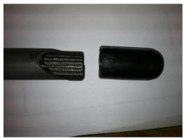
2. Once the bolt is loose and the cover has been removed, insert the handlebars. Twist the handlebars so that it is perpendicular to the frame.
